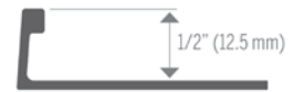
2152 1/2" X 8" TILE EDGE. SKU 68-2152-XX | SIZE 8' COLOR Available in Titanium, Satin Clear, Satin Black & White
