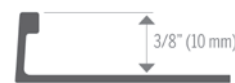
2151 3/8" X 8" TILE EDGE. SKU 68-2151-XX | SIZE 8' COLOR Available in Titanium, Bright Clear, Satin Clear, Satin Black, Matte Black & White
