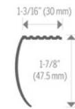
2193 1 7/8" DROP STAIRNOSING SKU 68-2193-XX | SIZE 1 7/8" x 12' COLOR Available in Titanium, Silver, Gold & Matte Black
